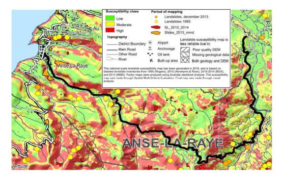
Figure 5 Landslide susceptibility map showing the road alignment (extract from CHARIM)
