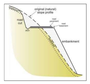
Figure 48 Road construction in mountainous terrain. The material excavated in the road cut is used as fill for the embankment.
